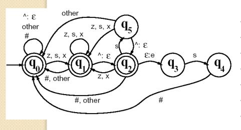
How would we represent this in NLTK? from nltk\_contrib.fst import fst f = fst.FST('pluralize') f.add\_state('q0') f.initial\_state = 'q0' f.set\_final('q0') f.add\_state('q1') f.add\_arc('q0', 'q1', 'z', 'z')
